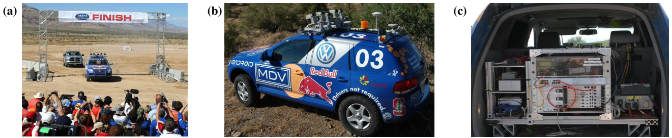
Figure 1: (a) The robot shown at approximately 1:40pm on Oct 8, 2005, as it successfully completes the 132-mile course. (b) View of the car and the roof rack with sensors. (c) The computing system in the vehicle's trunk.
