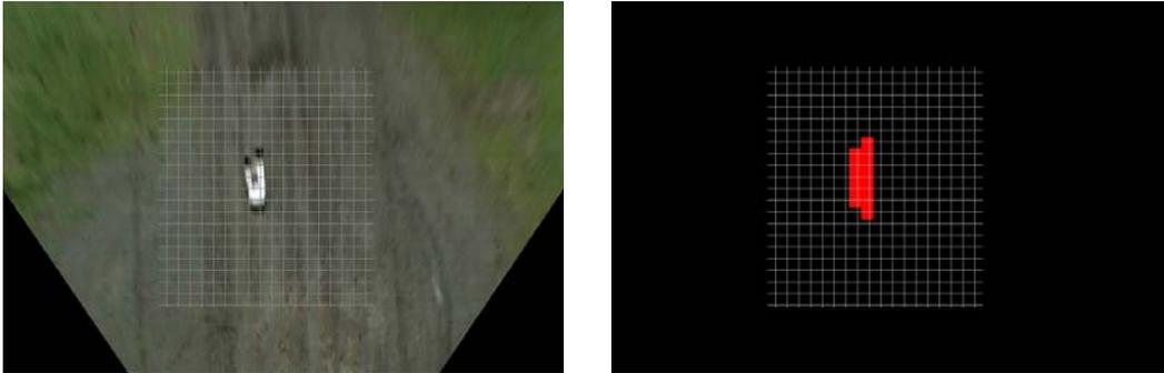
**Fig. 4.** Left: grid overlay on top-down view with object. Right: grid with red cells where object has been detected.
