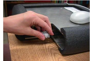
**Figure 1.** The Moose, a haptic interface [from 12].
