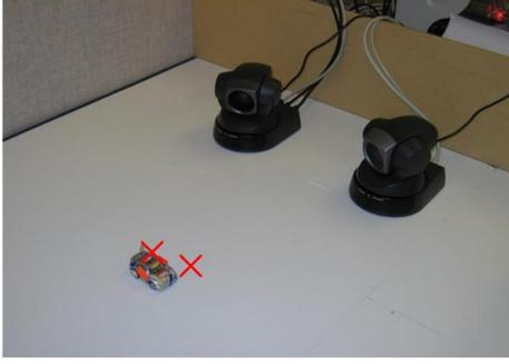
Fig. 6. The experimental setup with two cameras is shown in the picture. The crosses are the measured position of the object by the cameras.
