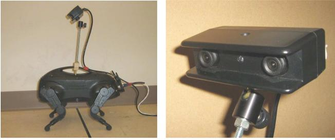
Fig. 3. (left) LittleDog robot equipped with a Tyzx DeepSea stereo camera. (right) Closer view of the camera.
