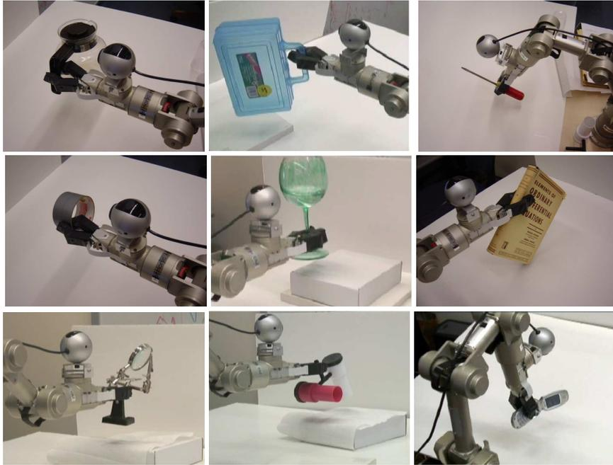
**Fig. 6.** The robotic arm picking up various objects: jug, box, screwdriver, duct-tape, wine glass, book, a chip-holder, powerhorn, and cellphone.
